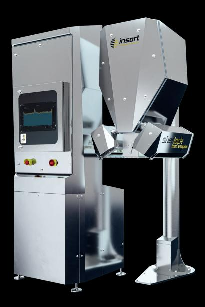
The Sherlock Food Analyser is the first choice when it comes to analysing dry matter and other quality parameters, non-destructively, in real time.
