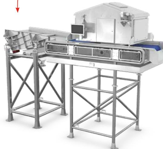
PeelGuard® also provides up-to-date information about the quality of the raw materials used. Additionally, the PeelGuard® can continuously optimize the settings of your steam peeler with data from the control process. The PeelGuard® thus ensures a constant, optimal peeling yield. ■
