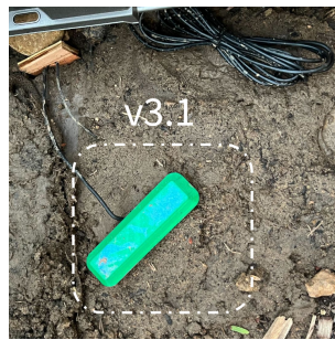
Fig. 19. Top view of the v3.1 cell buried outside in an irrigated residential yard. The v3.1 cell is covered with a 3D-printed cap that prevents debris from entering while allowing for airflow.
