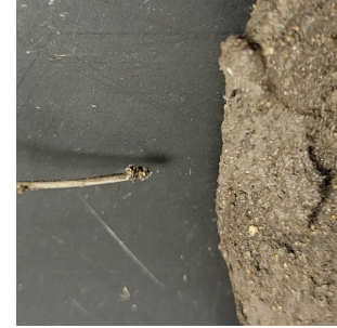
(b) Dirty/disconnected wire.
