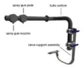
>>> Typical spray gun assembly inside the spray pod (access cover removed)
